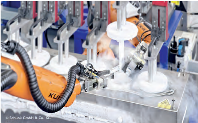
In the nitrogen bath, valve guides and seats are handled by two PGN-plus universal grippers. (Photos: Schunk)
